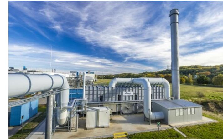
RTO units with two, three or more chambers are used in all industries that emit VOCs. They can be used for a wide concentration range and operate very economically, even without additional external heat recovery.
