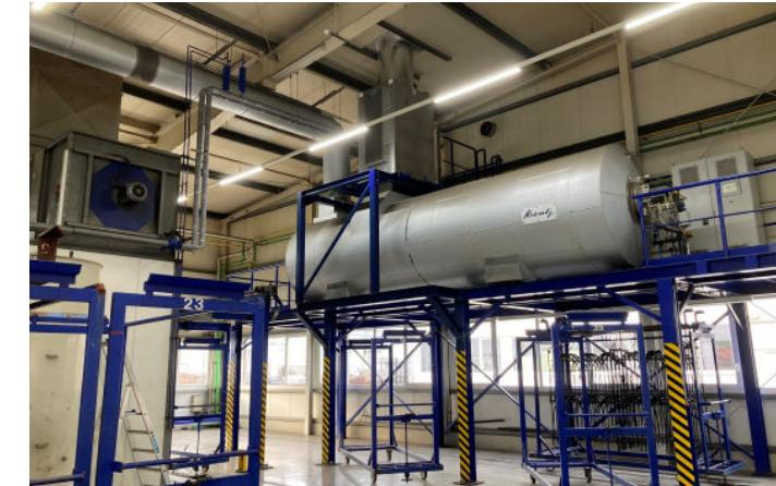
The compact thermal recuperative oxidisers are the preferred units for the cleaning of industrial exhaust air with high concentrations of VOC's which occur mainly in printing, coating, laminating and impregnating processes.
